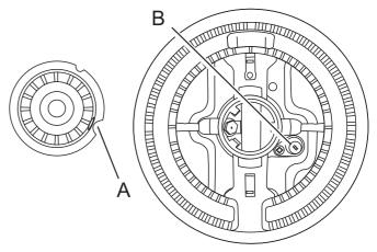
A electrode notch B ignition electrode
